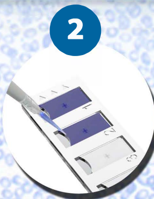
2 Pipette 20µl of sample into a QuadSlide™ chamber
