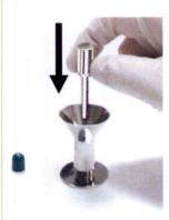
**4.** When the required quantity of powder has been put into the funnel, use the tamper to compress filling material into capsule body.
