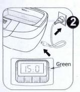
Insert one side of the detachable cord into the body of the machine and connect the plug to the socket. (See picture). Once the unit is plugged in, the green LED light on the right side of the control panel will turn on. The unit is now in standby mode.
