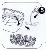
Pressing the OFF button for more than 2 seconds will turn the display off and put the unit in standby mode. When the cleaning is finished, unplug the unit and open the lid, then take out the items. At last, pour out the water from the stainless steel tank and wipe it dry.
