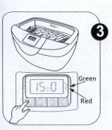
Press the "ON" button to start cleaning while the green indicator light is on.
