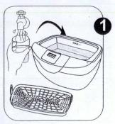
**Open the lid**, put the items to be cleaned on the tray and put the tray in the tank.
