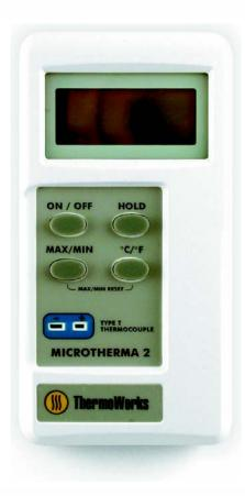
Type T thermocouples.  $\pm 0.2^{\circ}$ C meter accuracy. Self-calibrating circuitry. Includes Hold, Max and Min functions. Switchable  $^{\circ}$ C or  $^{\circ}$ F
