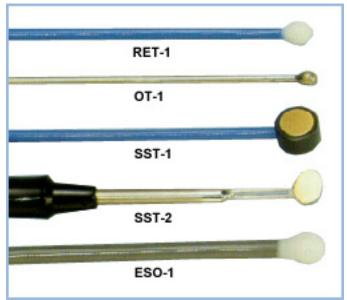
**RET-1** - Rectal probe for humans, neonatal, rabbits, and larger animals. Flexible, vinyl covered, soft tipped. Does not cause discomfort. Max. Temp. 90°C. Time constant 5.0 secs. 5 ft. lead. Isolated.
