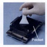
5. When all the holes have capsule bodies in them, pour out a pre-measured quantity of powder. Spread the powder with the Spreader. Push the excess powder to the Pocket.
