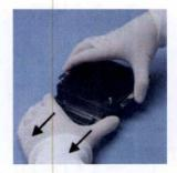
7. Slowly pull out the Spacer Plates one at a time. Hold Capsule Holder with both Handles as you pull out each Spacer Plate and then gently let it down.
