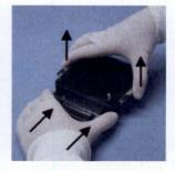
2. Lift the Capsule Holder using the 2 handles and push both Spacer Plates all the way in and under the capsule holder.
