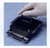
6. Use the Tamper to pack powder into capsules. Spread remaining powder as in step 5 for proper fill weight.
