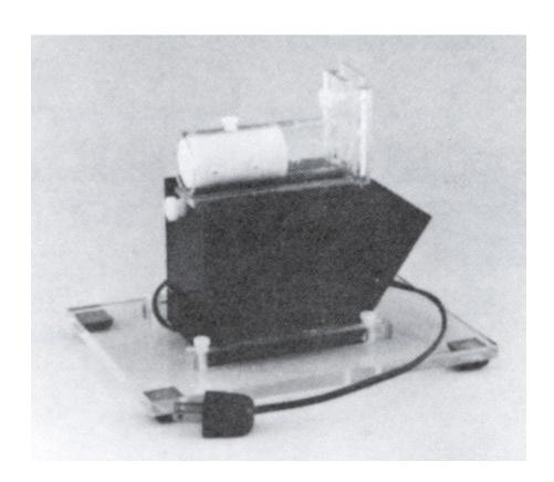
Efficiently illuminates and warms a mouse tail for easy injection or bleeding. Sliding doors keep mouse gently restrained. Each unit comes with a restraining tube and illumination source.
