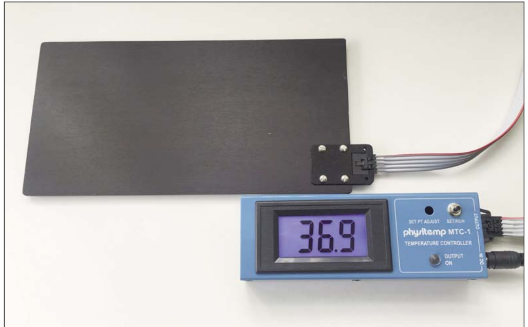
MTC-1 Micro Temperature Controller set-up with HP-1M Animal Warming Plate
