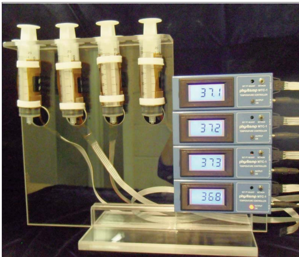
Four MTC-1 Micro Temperature Controllers set-up with perfusion syringes.
