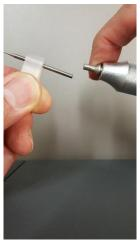
To insert burrs, always place your index finger firmly on the chuck's dome, next insert the burr to the opening and press it in. The tip of the burr should stick out about 20 mm
