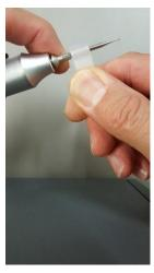
To remove the burrs, place your index finger firmly on the chuck's dome, insert the removal tool as shown, then pull the burr out. If the metal chuck opening becomes loose-fitting, use a small pair of fine pliers, to squeeze tight the opening. If you over pressed the opening of the metal chuck, then use the other end of the burr to insert and re-open it to the burr's diameter
