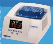
It's compact footprint incorporates an intuitive control panel with a large multicolor display, which allows users to easily program and view temperature, time and speed settings. Eight interchangeable aluminum blocks accommodate PCR plates and a variety of common tube sizes, including a combination block that hold both 0.5mL and 1.5mL tubes. Designed to meet the high-paced demands of today's lab, the exceptional performance of this product make it an essential part of your daily research.
