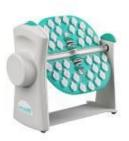
To create a Tumbling motion for your samples, turn the Rotisserie plates so the samples are in a "Vertical Mixing Position"
