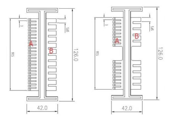
Small teeth (Side A): W= 3mm D=1mm. For a typical 0.5cm thick gel, the volume= $3*1*(5-1)=12\mu$ l
