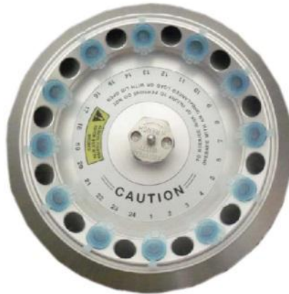
Figure 1. Loading the rotor to achieve balance
