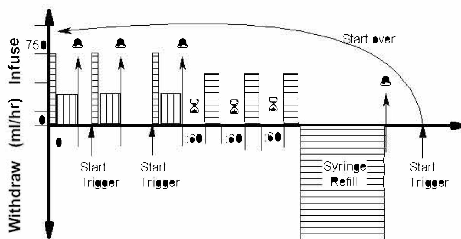
A more complex dispensing example, this Program contains different pumping requirements, including dispenses with multiple pumping rates. The first set of 3 dispenses drops down to a lower pumping rate during the dispense. When each dispense is completed, the buzzer beeps to alert the operator, then the pump waits for a start trigger before starting the next dispense.
