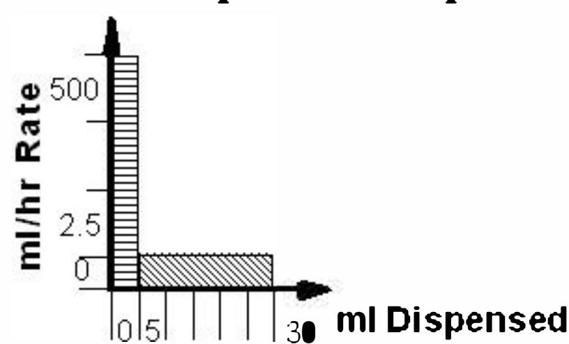
Infuse 5.0 ml at 500 ml/hr, then infuse 25.0 ml at 2.5 ml/hr. Then stop the pump.
