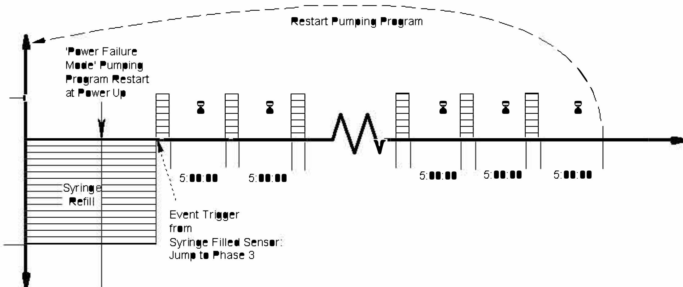
The following is an automated dispensing Program for a BS-8000/9000 syringe pump equipped with a 'Syringe Filled Sensor' attached to the TTL I/O connector, and a valve system to refill the syringe from a reservoir. It is also assumed that the 'Power Failure' mode is enabled.
