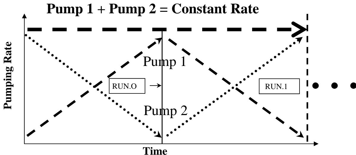
Maintains a constant total flow rate between 2 syringe pumps. A gradient (Linear function) dispensing function is programmed into the Master pump. The secondary pump will be automatically programmed with the inverse of the Master pump's gradient function. The sum of the two pump's flow rates will be a constant. Both pumps will increase and decrease pumping rates in tandem.
