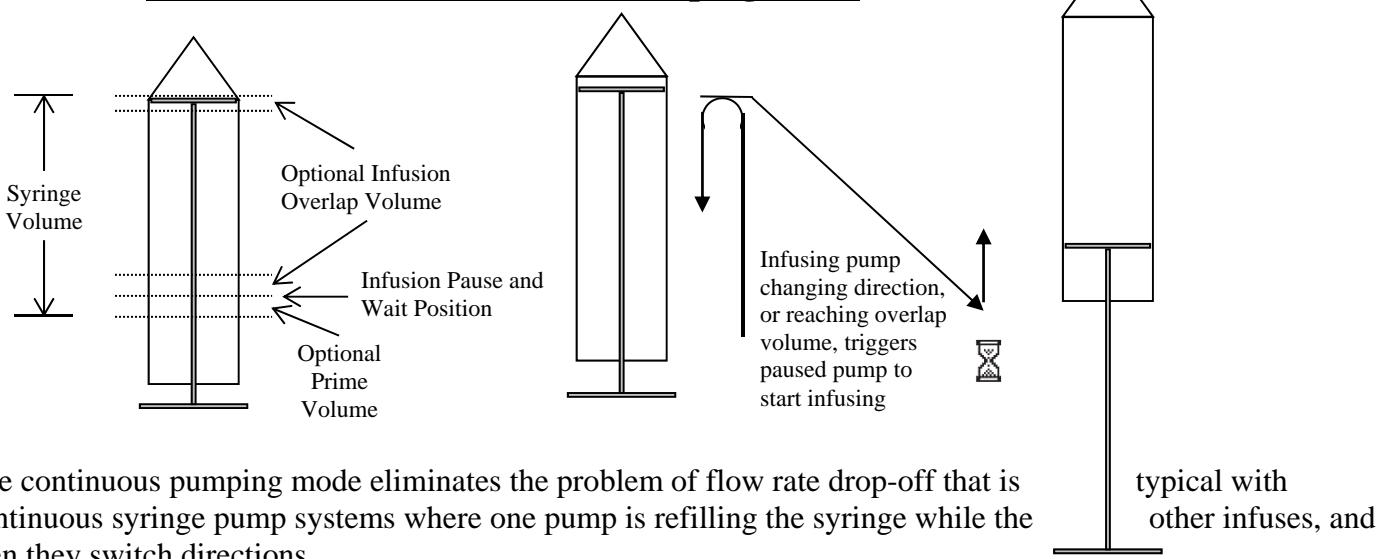
The continuous pumping mode eliminates the problem of flow rate drop-off that is continuous syringe pump systems where one pump is refilling the syringe while the then they switch directions.
