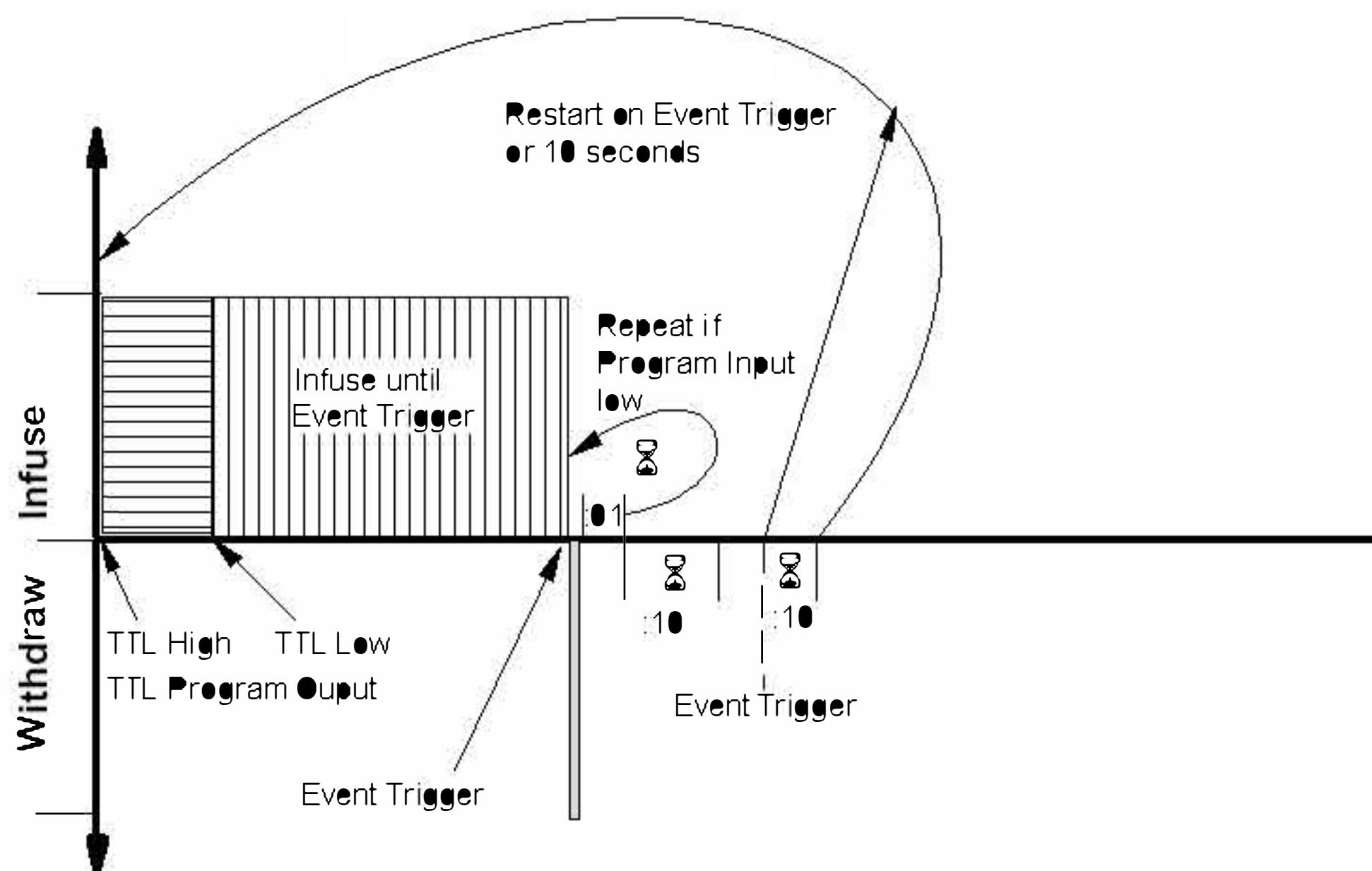
This example demonstrates a complex interaction with external equipment, such as synchronizing with another syringe pump. The Program includes a variety of interactions with external equipment, which demonstrates the various control possibilities of the BS-8000/9000.
