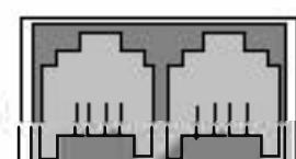
On the rear of the pump are 2 square RJ-11 ("phone jack" style) sockets. Connect the RS-232 cable into the socket labeled "To Computer". Connect the other end to the serial port on the computer, or other control device. Turn power off to the pump and the computer before connecting cables.
