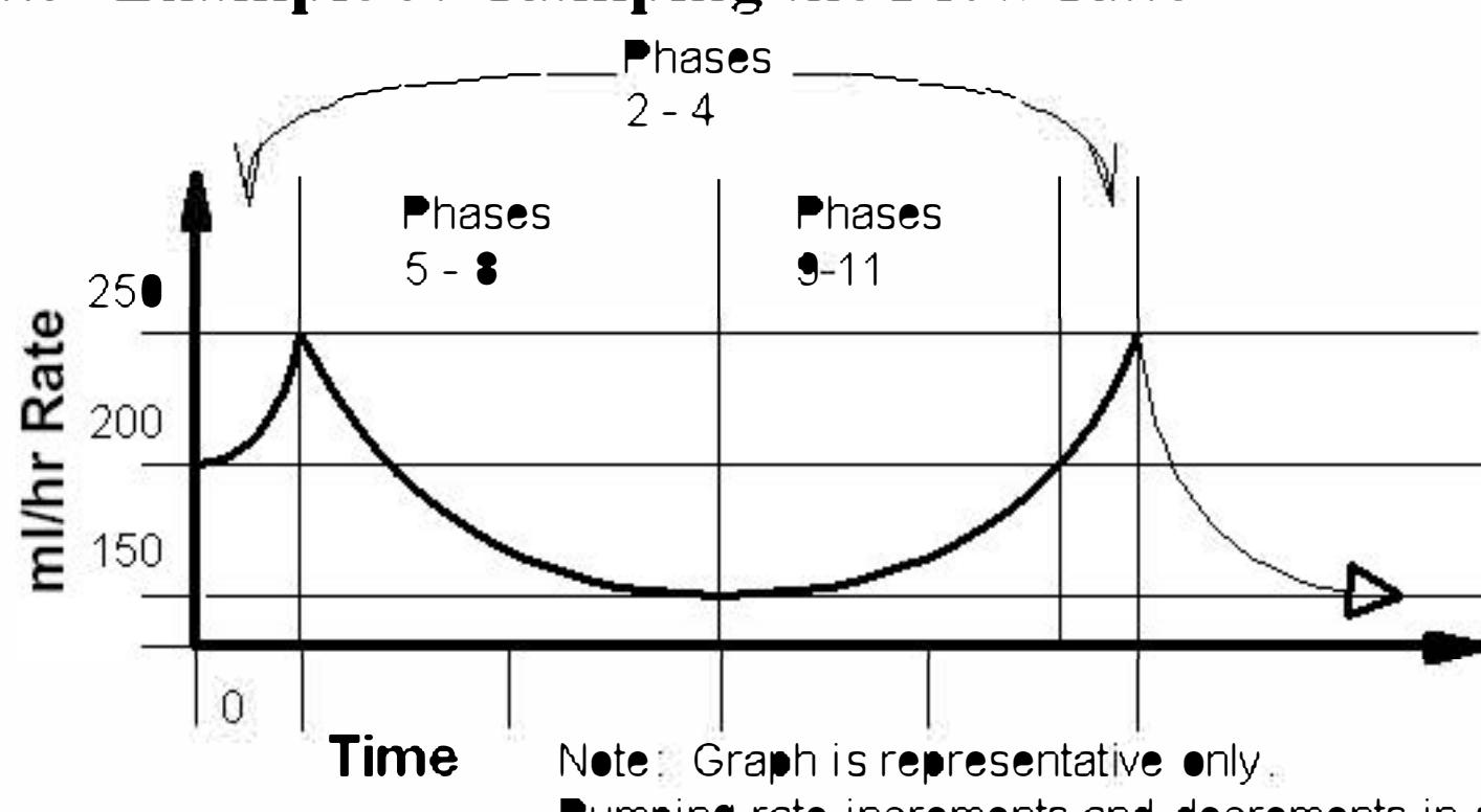
Continuously ramp up and down the pumping rate. Starting at 200 ml/hr, the pumping rate will increment to 250 ml/hr in 1.0 ml/hr steps after every 0.1 ml has been dispensed. Then the pumping rate will decrement to 150 ml/hr in 1.0 ml/hr steps after every 0.1 ml has been dispensed. Finally, the pumping rate is incremented back to 200 ml/hr in 1.0 ml/hr steps after every 0.1 ml has been dispensed, then the process is repeated.
