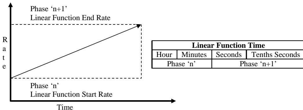
The Linear Flow Rate function is specified by using two Linear Functions **LINR**, in two consecutive Program Phases, defined by four parameters:
