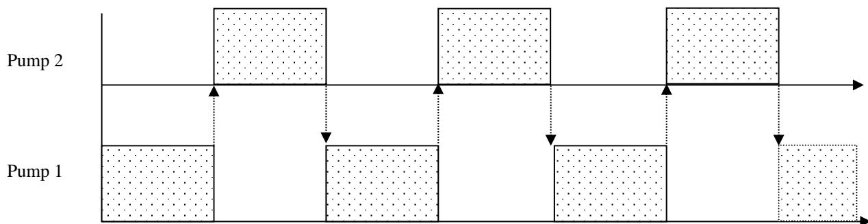
**Creates a semi-automated continuous infusion system using pre-loaded syringes.**
