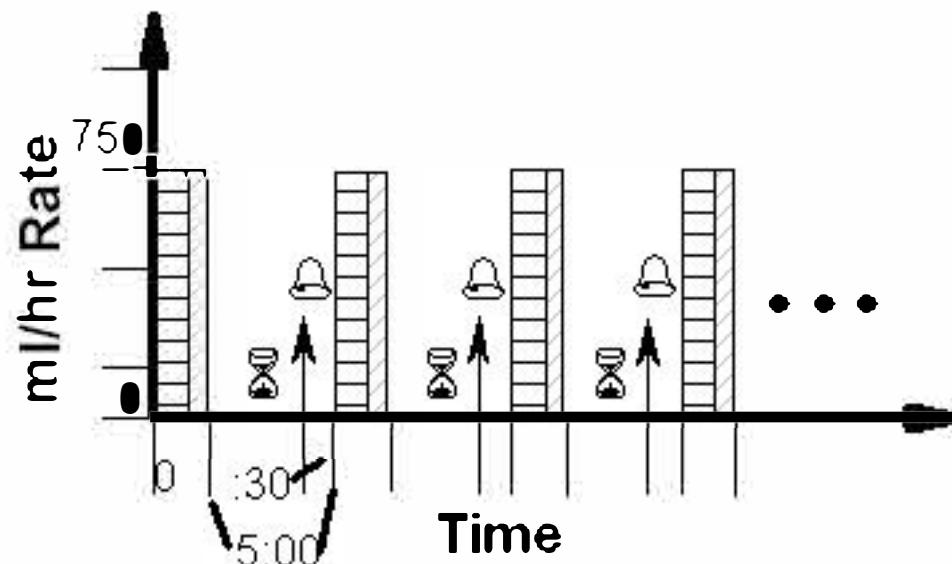
Dispense 2.0 ml with a 5 minute pause between dispenses. In addition, after each dispense, a volume of 0.25 ml is sucked back to prevent dripping. Also, 30 seconds before the end of the pause interval, a beep is sounded to alert the operator to prepare for the next dispense.
