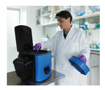
The Bullet Blender Gold models combine  $4^{\circ}\text{C}$  Cooling<sup>TM</sup> using dry ice, noise insulation to keep homogenization quiet, and extra-powerful homogenization.
