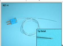
The new RET-4 Rectal probe for very small animals (neonatal mice). Flexible polyurethane sheath with smooth rounded tip (see inset). 36" long (can be made longer). Outside diameter nominal 0.032" (max at tip 0.04"). Time constant 0.18 seconds. Max temp. 140°C. May be sterilized by Gas (ETO), Gluteraldehyde solution or autoclave.
