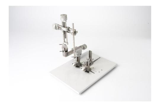
Like the classic Lab Standard<sup>™</sup>, the Ultra Precise, NEW Standard Stereotaxic Instrument has larger laser engraved Vernier scales (accurate to 10 um), 80 mm of ventral-dorsal, medial-lateral and anterior-posterior travel, absolute lock at 90° ventral-dorsal and brass-bushings for electrical grounding.
