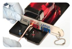
**Step 3**: Hold the tail across the v-groove, and starting with the smallest slot on the left, to the largest slot on the right of the Tail Gauge, determine the slot that fits the tail. The fit may be snug, but not tight. Do not use force.
