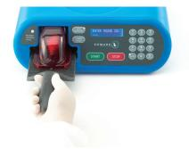
**Step 1:** Insert the Restraint Cartridge into the Applicator Machine.
