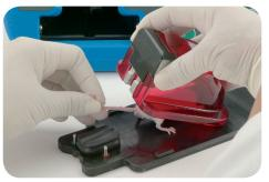
**Step 2**: Pick up a mouse by its tail and place it on the Restraint Cartridge platform. Depress the tail grippers on the red dome cover, position it over the mouse tail, and release grippers.
