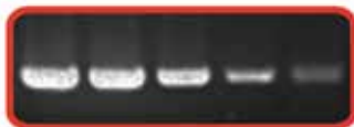
Gel image shows exceptional sensitivity of Accuris™ Hot Start Taq Polymerase with 405bp plant mitochondrial DNA. Amplification was performed with decreasing amounts of starting material, from 500ng to 31.25ng.
