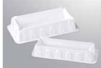
Designed for use with all multichannel pipettes. Standard 4 channel, 8 channel, 12 channel and various special purpose pipettes are all compatible with these disposable polystyrene reservoirs. To facilitate easy, dripless pour-off of unused reagents and solutions, all versions have indented "spouts" in each corner. Bottoms are formed with a sharply tapered "V" shape to minimize waste and reagent consumption. Packed in environmentally friendly packaging.
