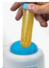
of 2800rpm, the Vornado instantly vortexes even the largest samples, including nearly full 50 ml tubes. Despite its powerful motor, Vornado has a footprint of less than 4" x 4", allowing it to fit on even the most crowded bench.
