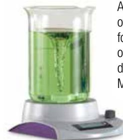
Advanced magnetic coil technology drives spinning of stir bar maintaining continuous, constant speed for reproducible results. Magnetic coupling is optimized by using alternating current (AC) as its driving force strong enough to stir viscous solutions. Motor-less operation generates minimal heat ideal for stirring temperature sensitive samples and environments for long periods.
