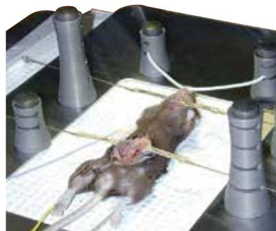
Magnetic fixators hold retractors and attach anywhere on the animal table. A push-button top operates multi-level locking jaws that grip wire or elastomers firmly.
