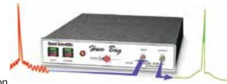
Cancels electrical interference in real-time, avoiding traditional problems associated with notch filters. Hum Bug constructs a replica of noise present on input signal and continuously subtracts replica from the signal as it passes through the instrument including biological activity even when noise characteristics evolve over time.
