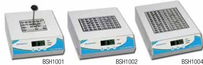
Accurate “set and walk away” digital temperature selection accurate within ±0.2°C. High grade aluminum block cavities are precision machined providing unsurpassed temperature transfer. Digital timer can alert user that a chosen time interval has timed out (timer does not turn heater off).
