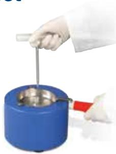
Freeze and process tiny tissue samples within a microcentrifuge tube. Mortar is suspended above a stainless steel cavity which holds liquid nitrogen and is nested in a heavily insulated blue polyethylene housing.
