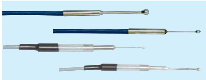
For fast intermittent measurements. The isolated sensor can be used with monitoring equipment where electrical interference from other electrodes may be present. Reinforced strain relief for applications where probe is in more frequent use. Smooth ball tip, 1" long stainless steel shaft, 0.059" dia. 0.125" tip diameter, 5' lead length. Time constant 0.8 secs.
