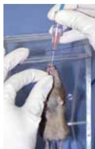
Using a small core fiber optic as both the stylet and guide wire, the FOS provides enough rigidity for applying mechanical force while remaining flexible enough to traverse convoluted paths. Light can also be delivered through the stylet/guide wire, enabling the user to illuminate the discrete places in the oropharynx directly where needed.
