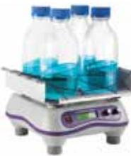
Allows user to create matrix for vessels of all shapes and sizes with hi-lo platform and bungee cords. Instantly adjusts to weight load changes and unbalanced loads with no-stop electronic motor feedback allowing for truly reproducible results. Suitable for use in incubators (excluding CO<sub>2</sub>) and cold rooms within the stated temperature range.
