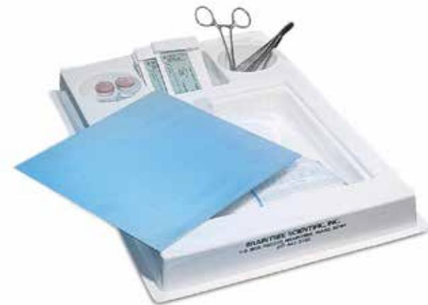
This compact operating board takes advantage of the Deltaphase principle to maintain animal body temperature during surgical or experimental procedures. An 8.5" square stainless steel operating surface lies in contact with an activated Deltaphase isothermal pad. The underside of the pad is insulated to provide a longer isothermal period. Molded wells are provided for sponges, instruments and anesthetic apparatus.
