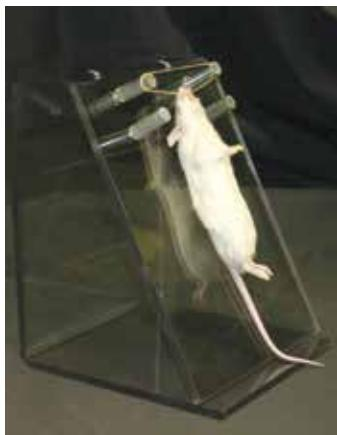
Constructed from durable polycarbonate, this platform provides the perfect stage for intubating mice and rats of all sizes.
