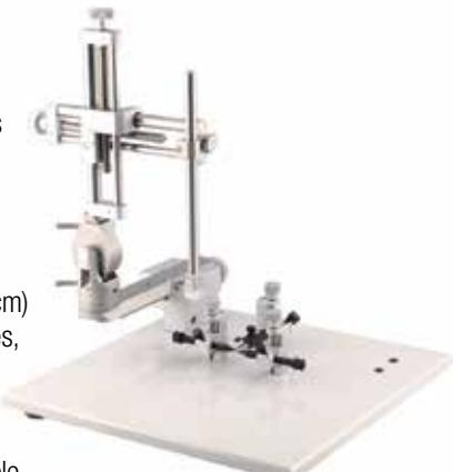
Includes 10" x 10" (25cm x 25cm) square base, 100 micron, 3-axes, left-hand manipulator arm, triple-point mouse and ear bars, snout clamp, and corner clamp probe holder. Also available as dual, ultra-precise, digital or motorized.
