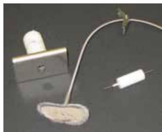
Constructed from lightweight stainless steel spring-coil, rodent tethers come complete with a crimped end for direct attachment to the rodent swivel (removing the need for potentially troublesome connection hardware). Jacket anchors comes ready sewn with silver woven fabric for added comfort and resistance
