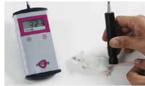
Optical dimension and position of IR sensor allows measurements on very small surfaces without allowing sensor to get wrong values arrived from integration of environment temperature. Allows **easy measurements even on mice tails** – with high accuracy and repeatability.
