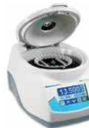
Touch-screen microcentrifuge offers high speed (up to 13,500 rpm/16,800 xg) and a unique Combi-Rotor™ with lid that accepts both standard microtubes (1.5/2.0ml) and PCR tubes/strips (0.2ml).
