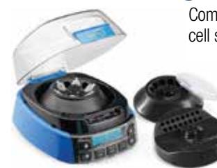
Compact centrifuge is ideal for PCR, microfilter cell separation, clinical and diagnostic applications, and HPLC protocols. Made of durable ABS with UV-resistant coating.
